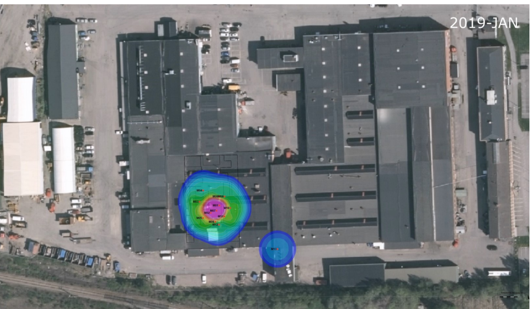
MIP XSD Sensor visualization of preliminary contamination delineation – Single source area
